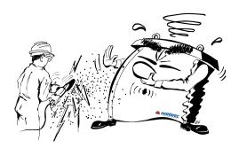
Do not use welding equipment, grinders or similar equipment close to the transformer unless they are surrounded completely with protective wrapping.
