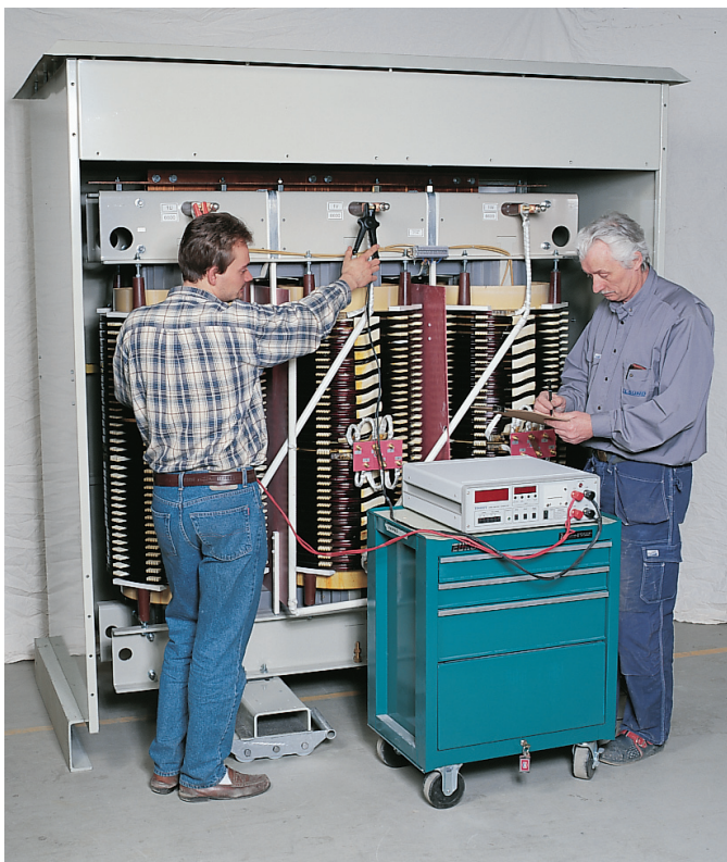
Test on a Noratel transformer. Testing is done by registering the maximum operating temperature, checking that the insulation is adequate and verifying specified losses and other values specified in standards and regulations.
