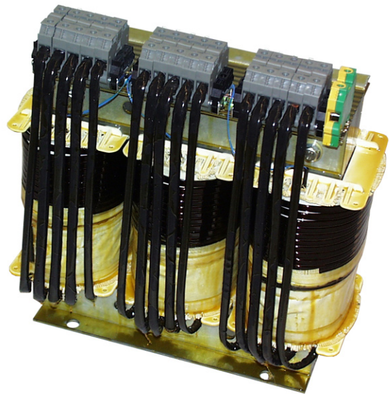
Three-phase autotransformer for motor start-up from Noratel. It is equipped with, among other things, thermistors for monitoring and disconnection in the event of a fault. The transformer can be supplied with a large number of tapings/adjustments for several stages if desired. Small overall dimensions versus high motor powers.
