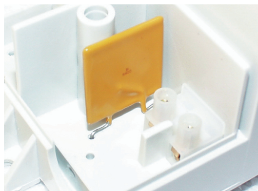
PTC mounted in an LF transformer
