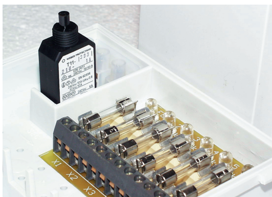
Miniature circuit-breaker and glass tube fuses fitted in transformer. The miniature circuit-breaker can be reset manually, whereas the glass tube fuses have to be replaced when they blow.
